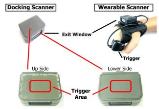
The touch sensor area is around middle of the scanner as drawing shown.
